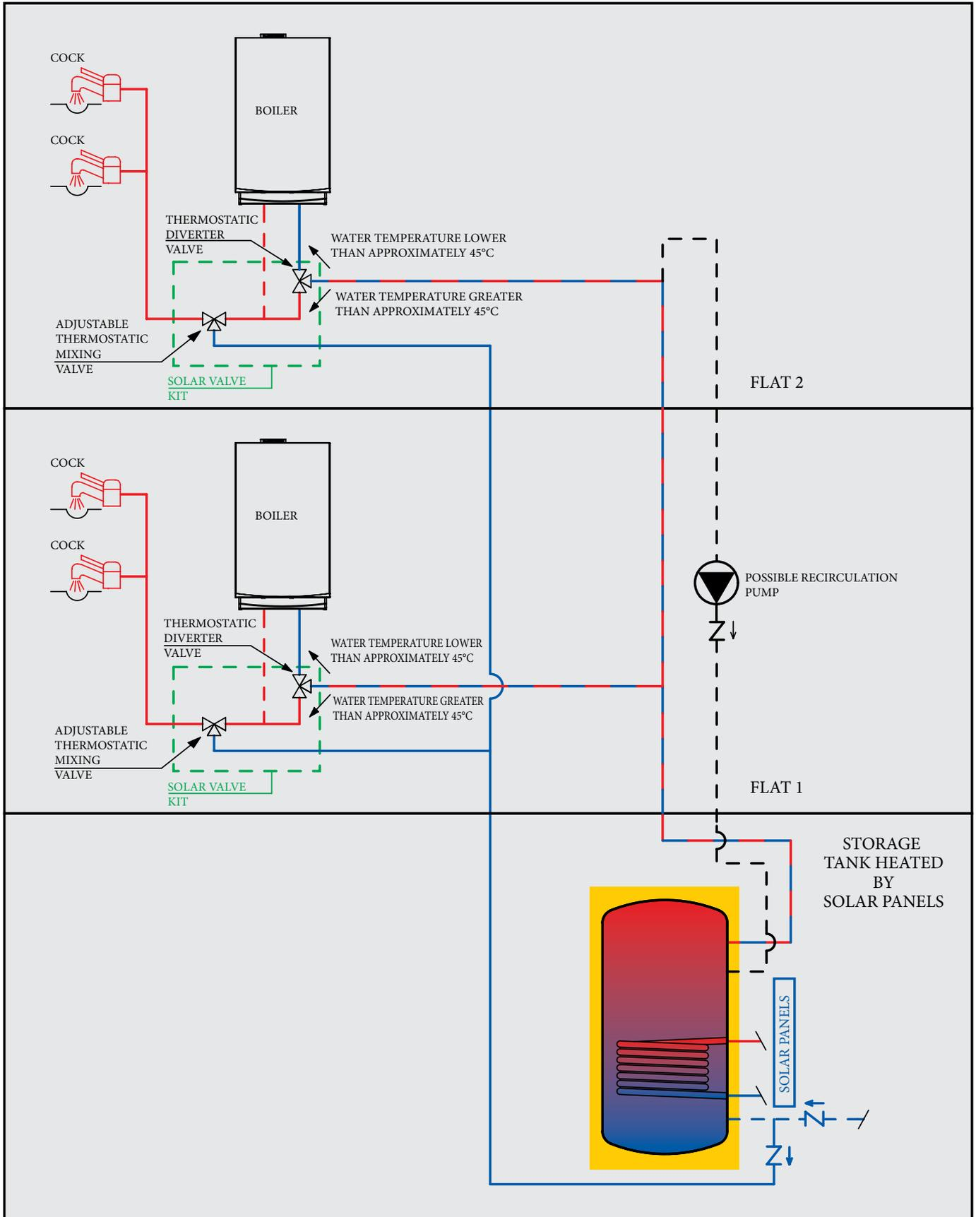
The system represented has the advantage that the centralised domestic hot water storage tank can be positioned in a common part of the building, as it has not particular installation restrictions (apart from structural ones) having no electric or gas supply.
