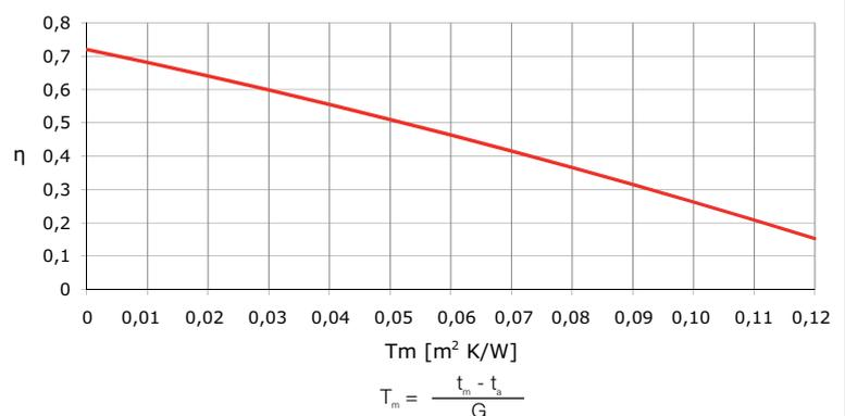
$t_m$  = average temp. in collector  $t_a$  = room air temp. G = total solar radiation intensity
