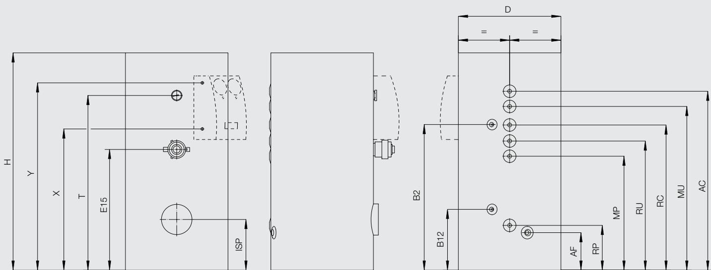
N.B.: while performing the connection, set up a drain fitting and an interception cock at the cold water inlet (AF) to facilitate maintenance operations.
