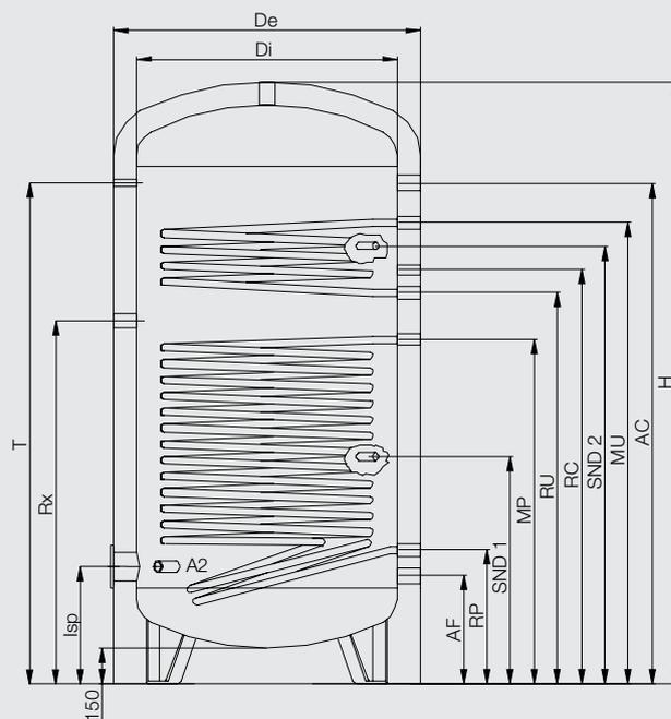
Dimensions of UB 1500 and UB 2000 litres
